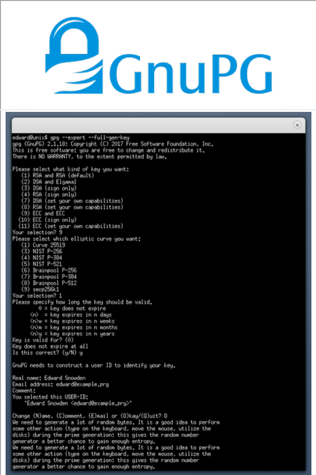
Key pair generation process in Unix terminal emulator
